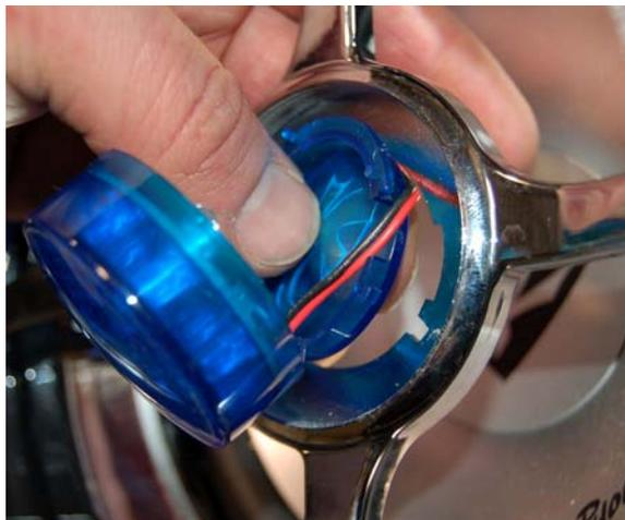
4. Remove the LED circuit board from the outer lens. The board is pressure fitted into this lens to stop any rattling so you have to very carefully remove it.
