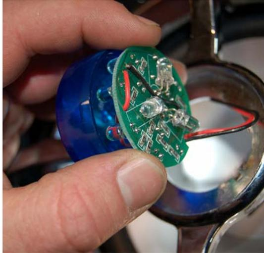
5. Replace the inner lens (red or white) lining up the lens with the Alignment notch ensuring that the wires are in the gap.
