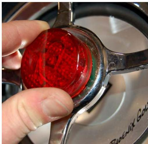
7. Be sure not to cross thread the bezel – It screws on with fine threads so caution is important.
