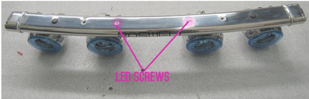
1. Align the new LED lens and tighten the two screws. Replace the assembly in the bar and align the top two screws.
