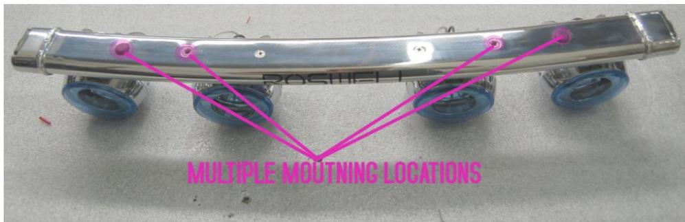
1. Remove the plug from the extra hole (C4 has 2 positions and C6 has 3) and attach clamp to new position.
